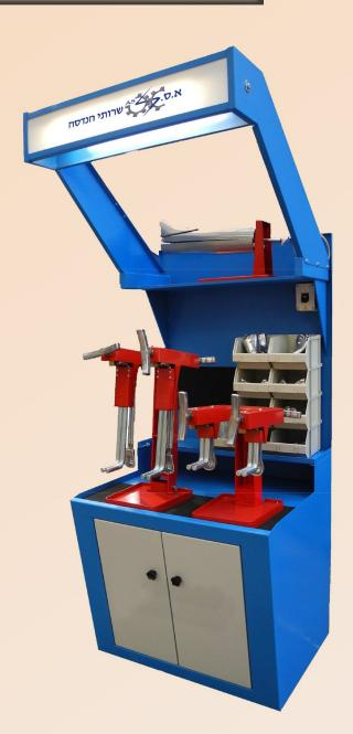
SHELF with 6 LASTS' JACK - working shelf endowed with a 6 lasts' jack and plastic drawers for material storage. It is also the ideal location for the Small Oven.
