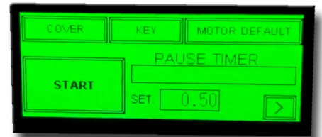
Electronic control panel supported by PLC System
